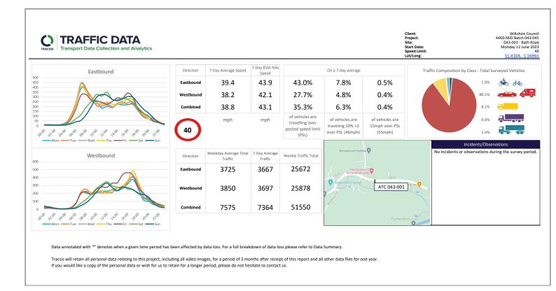
Speeds were recorded in front of The College over 7 days by 'double rubber line' sensors. The results need some explaining, but essentially within the 40mph zone where the test took place, just over 35 per cent of the motorists were found to be breaking the speed limit. But, crucially, the bulk of drivers were going no faster than an average speed of 43.1mph.
